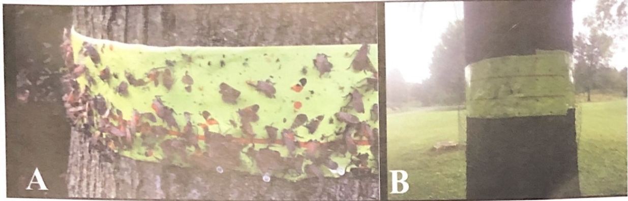
Figure 2. (A) A sticky band that has been cut in half to reduce the surface area and risk of vertebrate bycatch and (B) a sticky band that has been covered in a chicken-wire caging to prevent vertebrates from getting stuck on the band.
